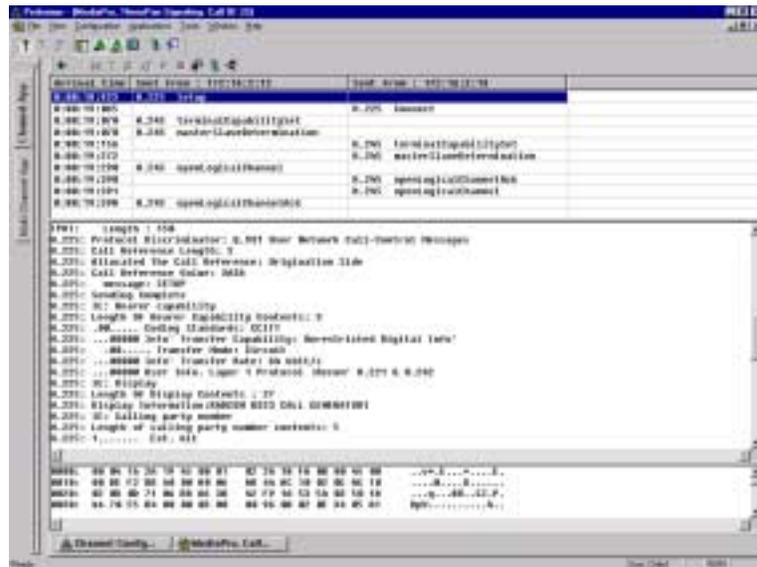
requires detailed decoding capabilities of all VoIP protocols. H.323 protocols use the ASN.1 notation while protocols such as SIP and Megaco use plain ASCII messages. Figure 3 shows the signalling decodes of a VoIP call and Appendix I includes a complete list of all VoIP protocols and their specifications.
