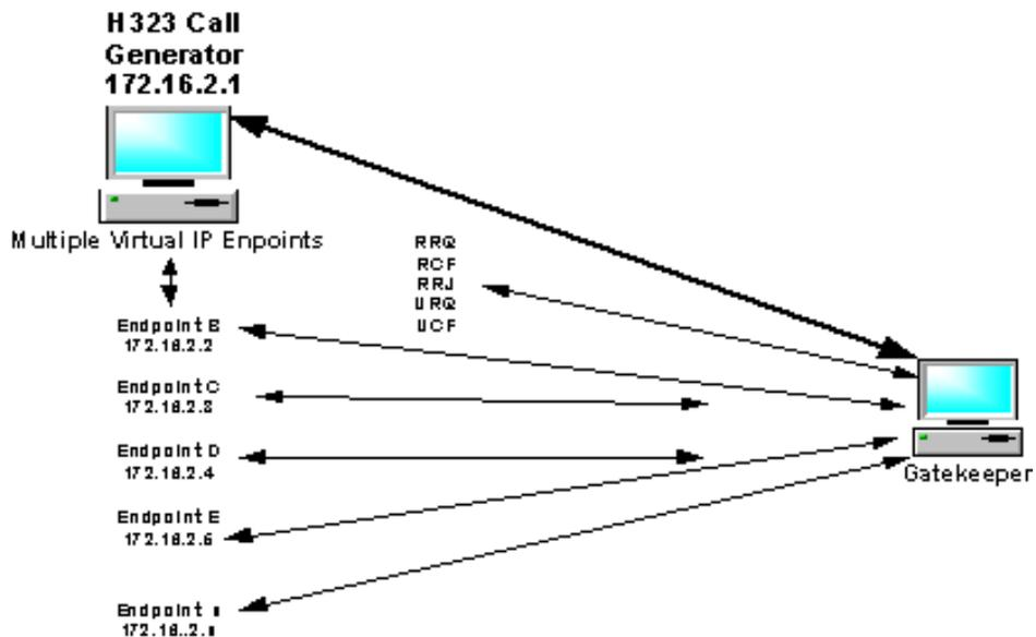
Figure 15: RADCOM's 323Sim emulates multiple IP phones
