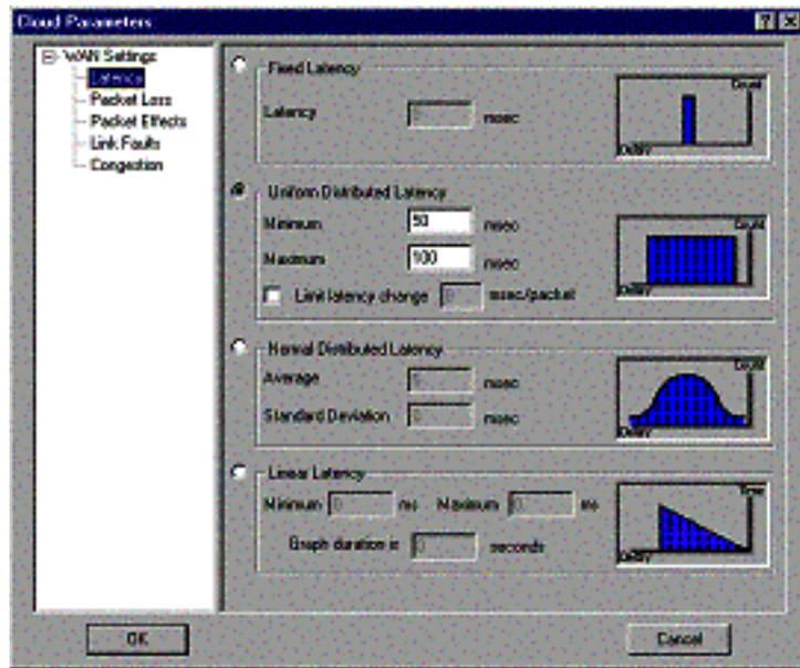
Figure 9: Latency emulation using NetSim
